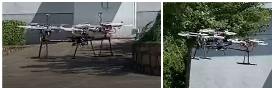
Figure 8. The IAP prototype maintaining a hover while changing its roll and pitch angles.
